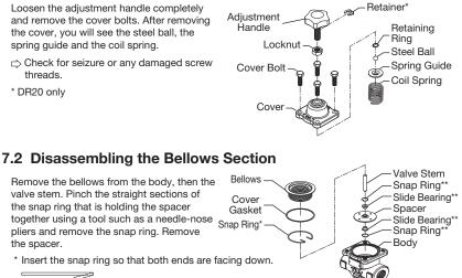
\* Insert the snap ring so that both ends are facing down.
