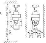
Leave sufficient space for maintenance, inspection and repair.
