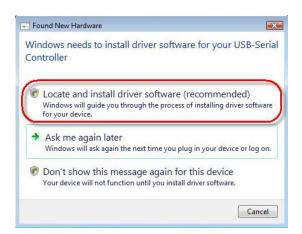
When [Windows needs to install driver software for your USB-Serial Controller] comes up, select [Locate and install driver software (recommended)].
