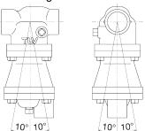
Make sure the product is installed with the raised TLV lettering on the body horizontal.
