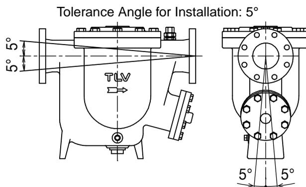
Make sure the product is installed with the raised TLV lettering on the body horizontal.
