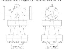
Make sure the product is installed with the raised TLV lettering on the body horizontal.
