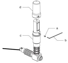
2. Once the cap is removed, turn the silicon-molded LCD display so that the LCD display is readable. After the adjustment is made, put the transparent cap back on and tighten the hex socket head bolt with a tightening torque of 0.5 N·m.
