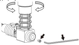
Adjust the counter body by twisting within 15° to the left or right. The angle should be adjusted based on the matching mark (a) and screw hole (b) on the body.
