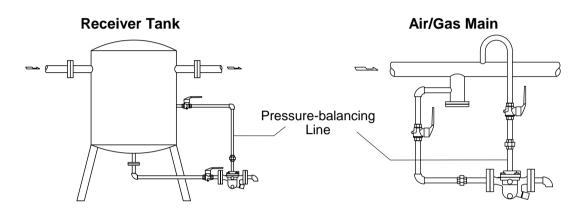
Connect the pressure-balancing line in the following manner:
