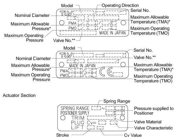
\*Maximum allowable pressure (PMA) and maximum allowable temperature (TMA) are PRESSURE SHELL DESIGN CONDITIONS, **NOT** OPERATING CONDITIONS. \*\*Valve No. is displayed for products with options. This item is omitted from the
