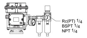
Integrated Filter: 0.3 µm + 5 µm
