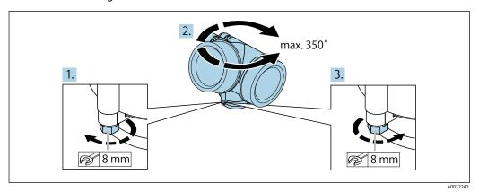
1. Release the fixing screw.
