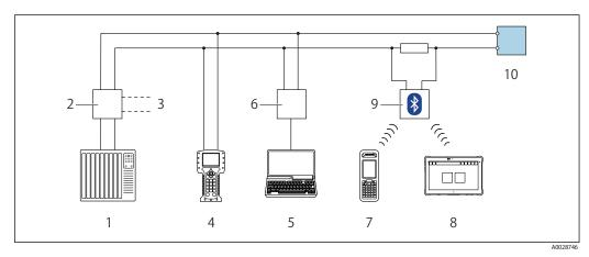
Fig. 18 Options for remote operation via HART protocol (passive)
