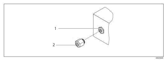
Fig. 27 Possible cable entries/cable glands
