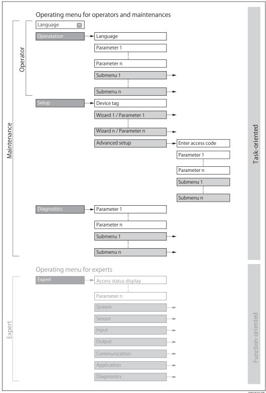
Fig. 16 Schematic structure of the operating menu
