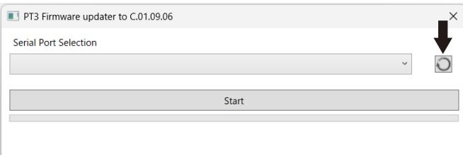
6. Confirm that USB serial device appears in the "Serial Port Selection" list.
