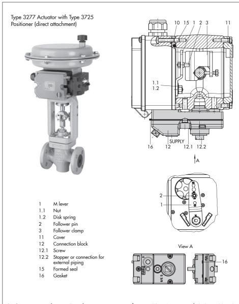
Fig. 9: Direct attachment · Signal pressure connection for Type 3277 Actuator with 240 to 700 cm<sup>2</sup>
