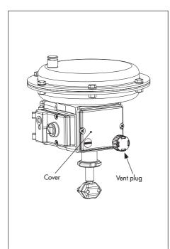
Fig. 7: Cover with vent plug when the valve is installed
