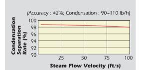
Separation rate (%) is given as: quantity of condensate discharged quantity of incoming condensate ×100
