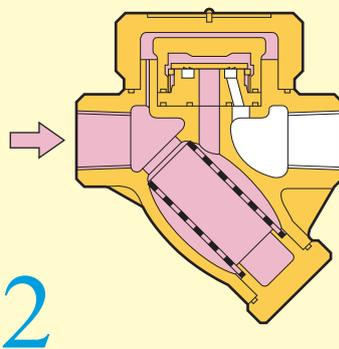
As temperature in the trap rises, the bimetal expands and releases the disc. The disc is forced downward by the low-pressure area created by the rapid flow of flashing condensate/steam below the disc, and the simultaneous high pressure in the pressure chamber above it. A steam jacket insulates the cap's pressure chamber from the radiant heat loss that could cause no-load actuation.
