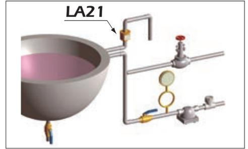
Note: • Inlet piping with no horizontal portion is recommended for water/air displacement. If there is a horizontal portion, make the pipe diameter of the horizontal portion larger than the vertical portion or make the horizontal portion as short as possible.
