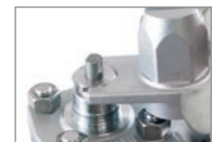
Tightening the gland retainer
