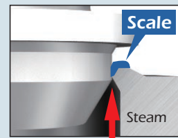
Scale is scraped off and flushed with steam by valve operation
