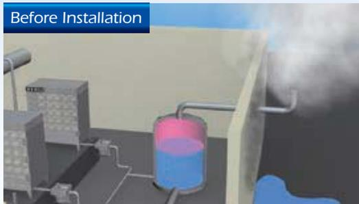
A condensate tank vented to atmosphere generates flash steam. Pressure cannot be applied to the tank, so conventional heat exchangers cannot be used.
