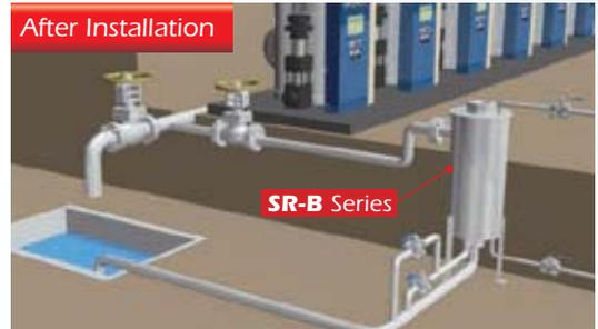
SR-B high-temperature waste water heat exchanger offers very little back pressure, handles blowdown and flash steam at the same time and exchanges heat with boiler supply water, raising its temperature. SR-B recovers heat and eliminates steam clouds simultaneously.
