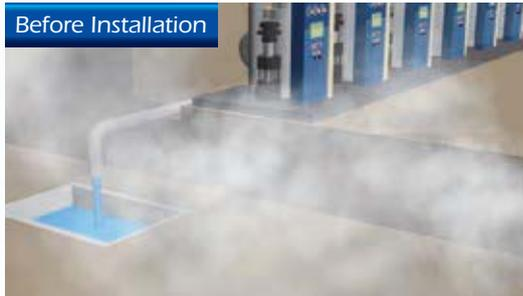
Boiler blowdown is hot and contains significant amounts of energy, however conventional heat exchangers are difficult to implement since they add back pressure to the boiler, therefore blowdown into a pit is more common.
