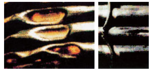
Water hammer damage to tubes and stays
