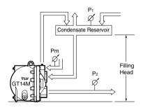
The discharge capacity is determined by the motive medium, motive medium pressure (Pm) and back pressure (P2).
