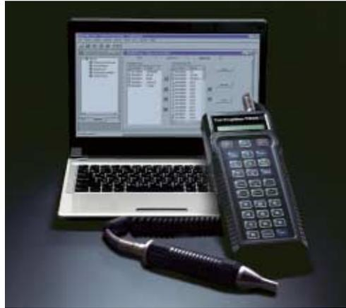
TrapManager allows users to determine the inspection route in advance. Then users can simply download this data to the TM5N-EX. When the inspection of one trap is complete, the number for the next trap to be inspected appears on the TM5N-EX display screen.
