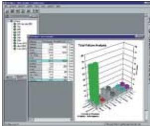
TrapManager processes data from TM5N-EX and then presents the results in a number of ways that users can select. For example, users can tabulate data for specific conditions and calculate the current failure state and rate based on available historical data.
