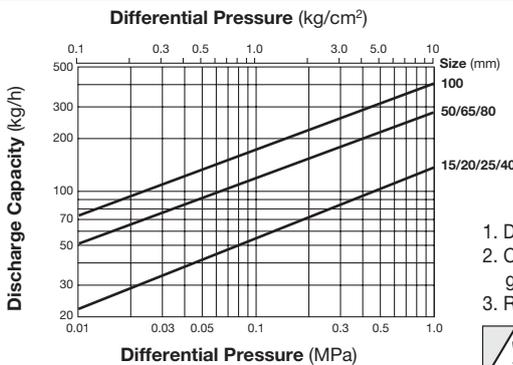
1. Differential pressure is the difference between the separator inlet and its trap outlet pressure.
