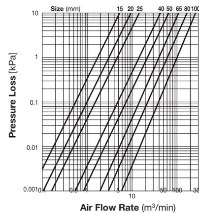
The pressure loss chart is based on an air pressure of 1 MPaG. For other pressures, multiply the air flow rate by the correction factor given in the table below. Use the result on the pressure loss chart.
