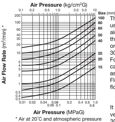
The chart at the left is used to determine the air flow rate through the DC3A. It is based on an air velocity of 30 m/sec.
