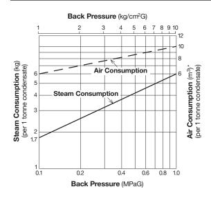
\* Equivalent consumption of air at 20 °C under atomospheric pressure
