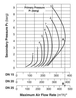
\* Equivalent flow of air at 20 °C under atmospheric pressure
