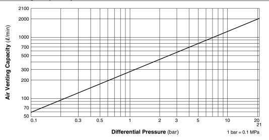
Differential Pressure is the difference between the inlet and outlet pressure of the air vent.
