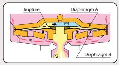
The pressure P3 approaches P2 and the valve plug is pushed up by the primary pressure P1 to open the valve.
