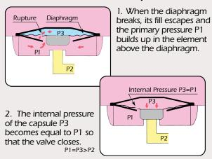
The closed valve causes condensate to accumulate.
