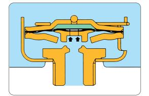
During start up of steam-using equipment while the capsule is still cold, the fill is in liquid state. The internal pressure is lower than the external pressure so that the diaphragm is pushed up to open the valve. Air, gases and condensate are discharged.
