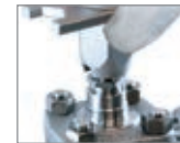
Adjusting the valve aperture
